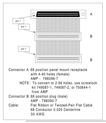
Converting Internal Wide to Internal Non-Wide (Type 2) The cable assembly for converting internal wide SCSI connectors to internal non-wide SCSI connectors is shown below:
